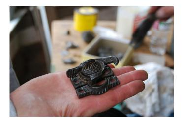
**And a final tip from the experts:** When starting to free up painted parts off a window of one of your Eureka California Victorian homes, try using an army knife to cut through the paint before you start removing any pieces. Then slowly and patiently start prying parts away using a small prying tool.
